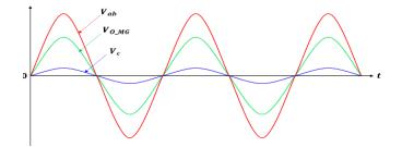
Figure 3. Main voltage waveforms of the S-PSI [1]
