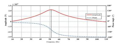
Figure 19. Frequency vs phase analysis of the S-PSI amplitude [1]
