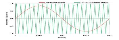
Figure 9. Reference sinusoidal and carrier triangular signal waveforms
