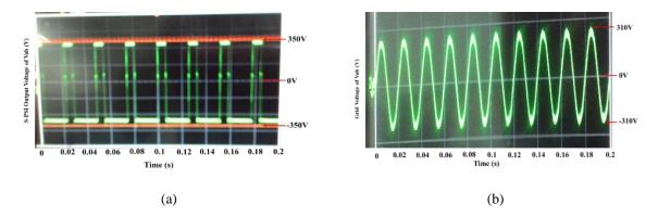
Figure 24. The Experimental voltage waveform for, (a) without filtering S-PSI, (b) with filtering grid
