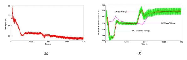
Figure 23. S-PSI for, (a) duty cycle waveform, (b) DC bus voltage
