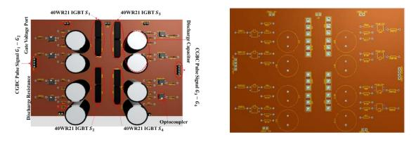
Figure 21. 3D PCB for S-PSI
