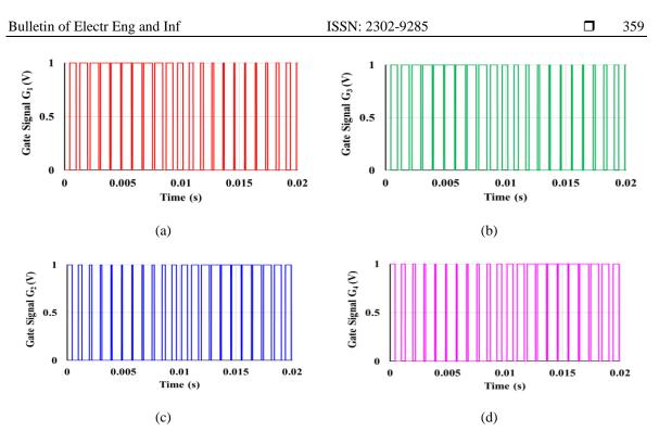
Figure 10. Separate comparator circuits signals  $(G_1, G_3, G_2 \text{ and } G_4)$  for SPSI
