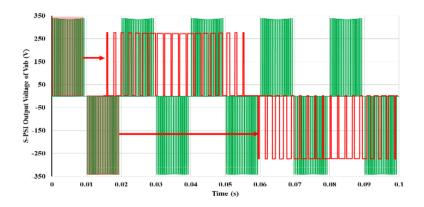
Figure 13. SPSI output voltage waveform without filtering condition [1]
