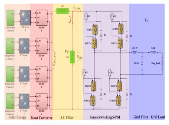
Figure 1. Proposed series switching SPSI circuit configuration [1]
