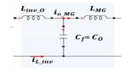
Figure 6. Equivalent circuit of grid couple lowpass LCL filter [1]
